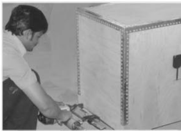
7. NAILING THE BOTTOM
